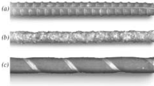
Fig. 5.1—Surface deformation patterns for commercially available FRP bars: (a) ribbed; (b) sand-coated; and (c) wrapped and sand-coated.
